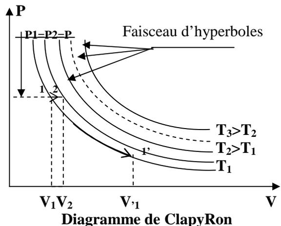
$$\left. \begin{array}{l} P.V_1 = r.T_1 \\ P.V_2 = r.T_2 \end{array} \right\}$$
